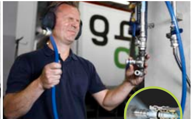
Standard - No anti-whip function
